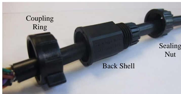
Figure 11 Cable with Sealing Nut, Back Shell and Coupling Ring
